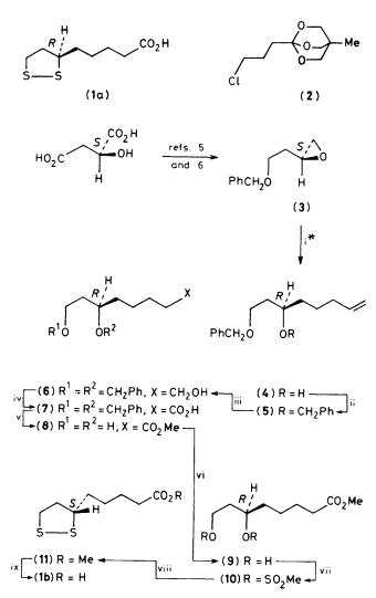
Scheme 1. Reagents: i,  $CH_2=CHCH_2CH_2MgCl$ ,  $Li_2CuCl_4$  (catalytic), THF; ii, PhCH<sub>2</sub>Br, NaH, THF; iii, HBSia<sub>2</sub>, THF, aq. HO<sub>2</sub><sup>-</sup>; iv, pyridinium dichromate, DMF; v, MeOH-HCl; vi, Pd/C, H<sub>2</sub>; vii, MeSO<sub>2</sub>Cl, Et<sub>3</sub>N; viii, Na<sub>2</sub>S, S, DMF; ix, aq. HO<sup>-</sup>. THF = tetrahydrofuran; DMF = dimethylformamide; Sia = PriC(Me)H<sup>-</sup>.
